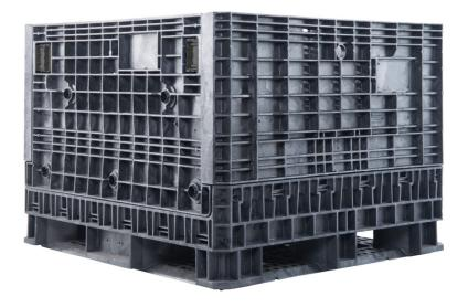
The heavy-duty Collapsible Bulk Container is used extensively by the automotive industry, as it meets the specifications of the Automotive Industry Action Group (AIAG). Unitized loads can be delivered directly to the assembly line for immediate part presentation, with no unwrapping or unbanding. Bulk containers collapse when empty for reduced return transportation costs and warehouse space savings. During storage and shipping these bulk bins stack securely atop each other.
